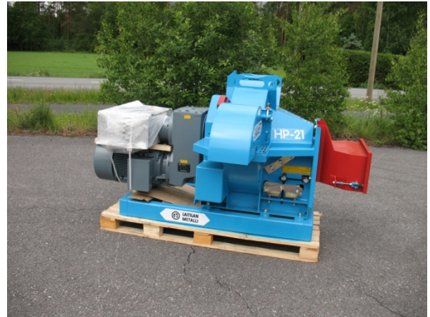
LS 21 IE chipper with gear drive transmission
