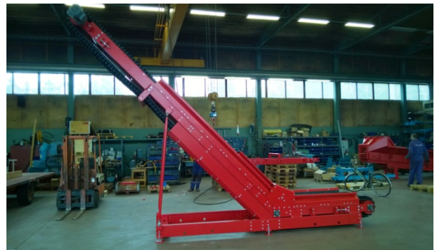
Chips Discharge Conveyor (GBBC 800/7350)
