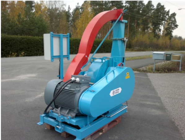
HS 21 IE chipper with V-belt transmission
