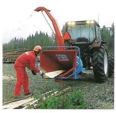
saplings, blocks, sawn surfaces and also frozen wood. The HS 21 A can chip up to 170 mm size wood and branches. Operational noise is comparatively quiet, but it is a good idea to use ear protectors because of noise from the motor.
